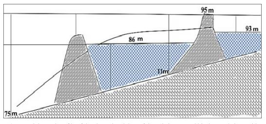
Fig. 5. Heights and profile of the channel and dam of the existing Repyakhivske pond along with the proposed dam of the storage reservoir, view from the left bank of the Komyshuvata River
